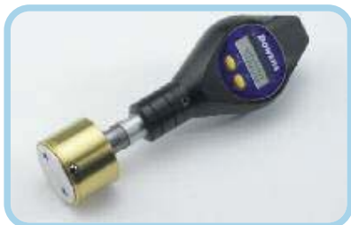
SmartPlug with TiN coated body
