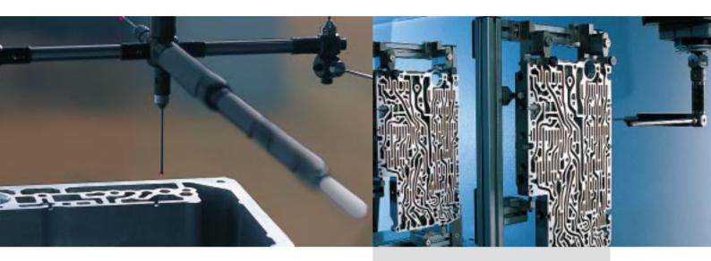
In the past, accuracy specifications of a coordinate measuring machine were related directly to the least favorable ambient conditions. If temperatures changed, you could never be sure just how precise your machine would measure.
