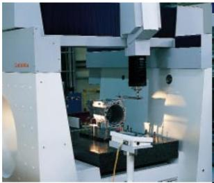
Most measuring machines are used exclusively in the metrology room. Traditional coordinate measuring machines require constant ambient temperatures and a vibration-free, clean metrology room. CenterMax® propels measuring technology into a new dimension.
