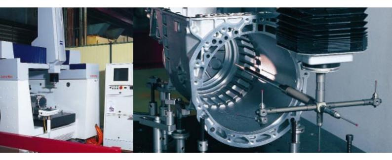
One of the primary demands made on a coordinate measuring machine to be used like a production device on the shopfloor: it must be resistant to environmental influences, much like a machining center. The solid construction and symmetrically arranged gantry axes ensure optimum vibration damping in milling technology and therefore also stable cutting processes. We have now borrowed this manufacturing design principle for our measuring technology.
