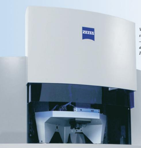
Whether micro-motors, microswitches or other tiny components – every micro-part can be highly accurately measured with the F25.
